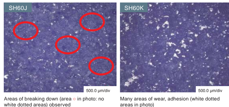
Fig. 1 Grinding wheel surface observation photo after grinding
