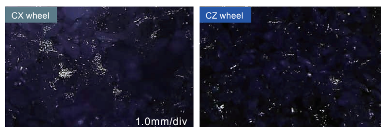
Fig. 3 Wheel surface inspection results after surface grinding.
