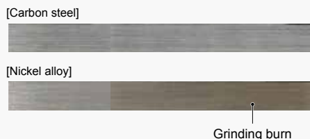
(b) Workpiece condition after grinding
